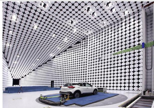
The importance of OTA propagation for the sensors essential for ADAS operation has intensified the need for measurement facilities with enhanced sensitivity, capability, and increased frequency coverage in a simulated real-world environment. A few of the more significant test techniques are presented along with a discussion on their challenges and merits.
